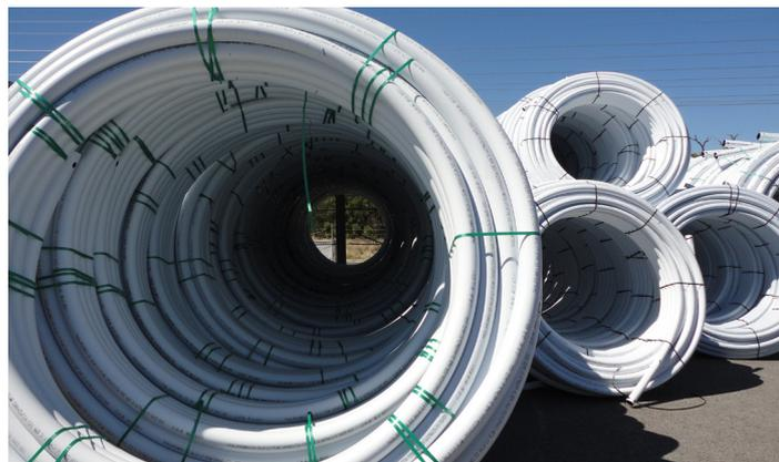
Other advantages over standard black pipe include a reduced temperature increase in fluids conveyed by the pipe, and by limiting operating temperatures a thinner pipe can be utilised.
